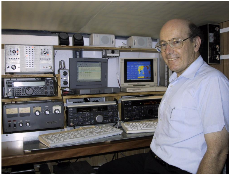
John Loftus VK4EMM, winner of the Frank Hine VK2QL Memorial Trophy and Oceania CW SOAB category, is ready for operation from his custom built trailer - affectionately known as "ComPort1". The two main radios are an FT1000MP and TS850. John's antenna farm includes three rotatable yagi beams on armstrong poles for 20m to 10m and multi-element wire arrays on the lower bands.
